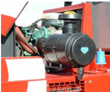
The air filter is easily accessible.
