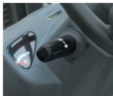
Finger-tip operation with the electric F/R lever
