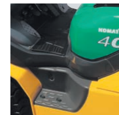
Improved design of engine hood and step
