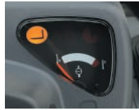
Lifting interlock lamp on the meter panel
