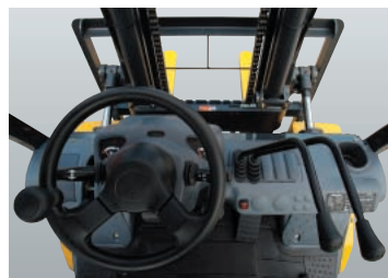
Finger-tip operation with the electric F/R lever
